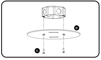
Using factory provided mounting tool set screw head distance on J-Box to prepare for fixture installation
