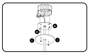
Lift fixture by the stem up to the attachment point and screw the mounting plate onto the J-Box. Complete installation by installing canopy cover to mounting plate.
