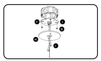
Hang fixture by attaching the mounting plate to the J-Box. Complete installation by installing canopy cover to mounting plate. Slowly lower fixture until supported by cables. Minor leveling can be achieved at J-Box gripper.
