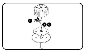
To install fixture, support in position just below junction box with lift.
