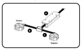
Remote driver must be installed within 100' from fixture. Use standard conduit to supply power to driver and from driver to separate low voltage positive and negative drops. Consult factory for custom driver installs.
