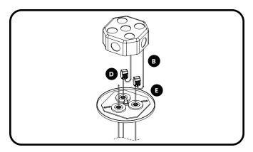
To install fixture, support in position just below junction box with lift\*\*. Make connection with the low voltage black and red wires from the driver to the corresponding air craft cables labeled positive or negative utilizing the provided 2-lever nut.
