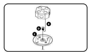
To install fixture, support in position just below junction box with lift. Make connection with the low voltage black and red wires from the driver to the corresponding air craft cables labeled positive or negative utilizing the provided 2-lever nut.
