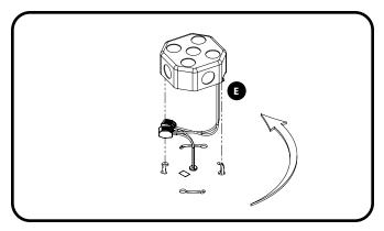
Hang fixture by lifting it onto preset mounting screws from step 2 and rotate and lock fixture into place. Note two mounting hole patterns for a large or small junction box.
