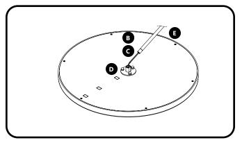
Push the low voltage positive and negatives wires exiting the fixture through the stem and thread the stem onto the adapter on the back of the fixture.
