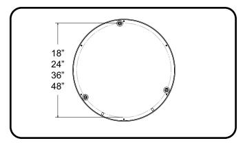
Junction Box mounting location; Ring fixtures require 3 J-Box at 120 DEG. on the circular pattern sized below.
