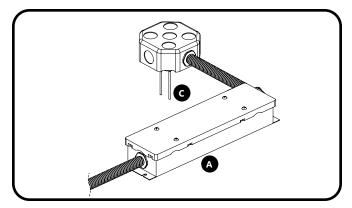
Remote driver must be installed within 100' from fixture. Use standard conduit to supply power to driver and low voltage positive and negative wires from driver to J-Box. Consult factory for custom driver installs.
