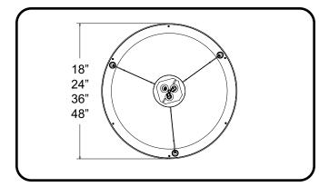
Junction Box mounting location; Ring fixtures require a J-Box mount
